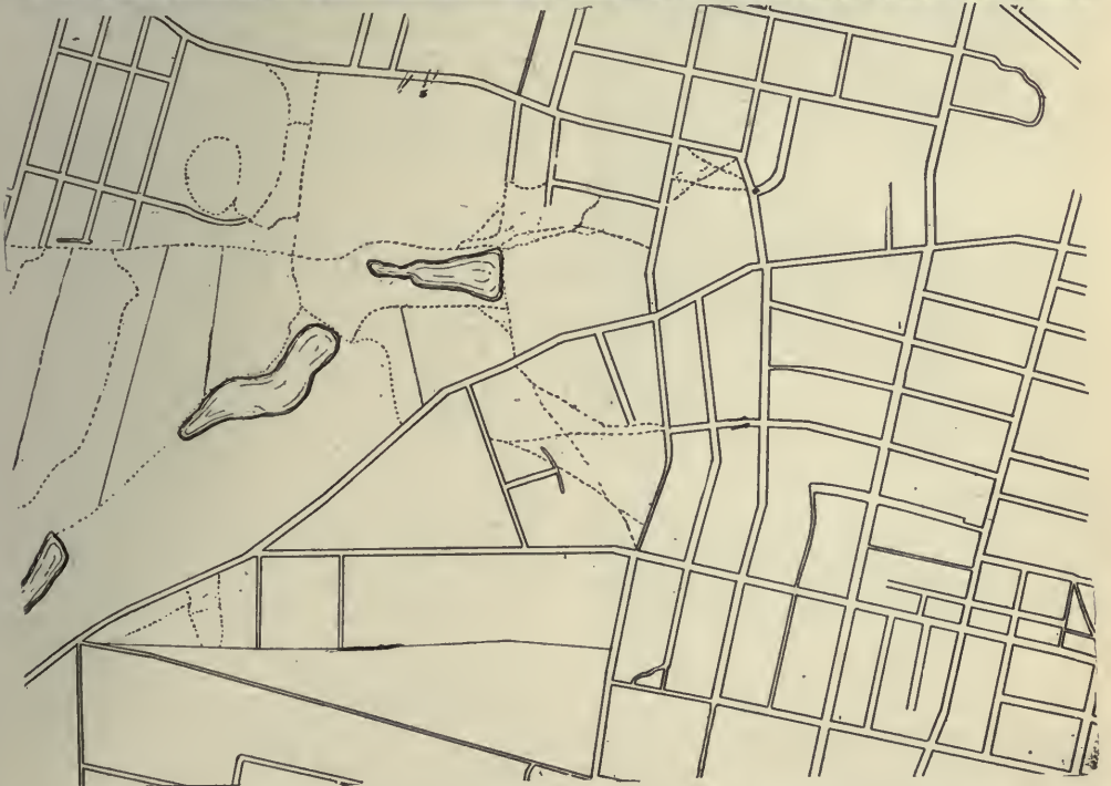
The photograph and line map above illustrate the advantage of an aerial photographic survey in the development of a city plan. The features of the photograph to be retained were inked in on the original; the photograph was then bleached, the inked lines only remaining. A study of both photograph and line map will be of great assistance to the city planner in determining the portions of the existing layout which should be retained, the connections and additions necessary to make a rational plan, and the topographical features which should be emphasized
